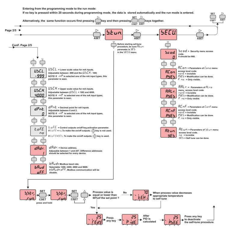
While holding  $\bigcap_{CSET}$  key, run message flashes. Then when  $\bigcap_{\triangle}$  key is pressed, self tune mode is entered if there is no probe failure. If process value is appropriate to begin self tune,  $r E d \mathcal{G}$  message flashes. Then press any key to see  $P \cdot d \mathcal{E}$ . message and self tune procedure begins.
