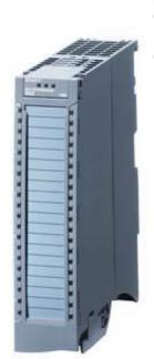
SIMATIC S7-1500, ANALOG OUTPUT MODULE AQ 8 X U/I HS 16 BITS OF RESOLUTION, ACCURACY 0.3 %, 8CHANNELS IN GROUPS OF 8, DIAGNOSIS, SUBSTITUTE VALUE 8 CHANNELS IN 0.125 MS INCL. INFEED ELEMENT, OVERSAMPLING SHIELD CLAMP AND SHIELD TERMINAL
