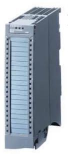
SIMATIC S7-1500, ANALOG INPUT MODULE AI 8 X U/I HS, 16 BITS OF RESOLUTION, ACCURACY 0.3 %; 8 CHANNELS IN GROUPS OF 8; COMMON MODE VOLTAGE APPR. 10V; DIAGNOSIS, PROCESSALARMS; 8 CHANNELS IN 0.0625 MS OVERSAMPLING INCL. INFEED ELEMENT, SHIELD CLAMP AND SHIELD TERMINAL
