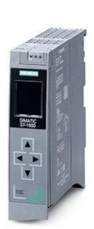
SIMATIC S7-1500F, CPU 1511F-1 PN, CENTRAL PROCESSING UNIT WITH WORKING MEMORY 225 KB FOR PROGRAM AND 1 MB FOR DATA, 1. INTERFACE: PROFINET IRT WITH 2 PORT SWITCH, 60 NS BIT-PERFORMANCE, SIMATIC MEMORY CARD NECESSARY
