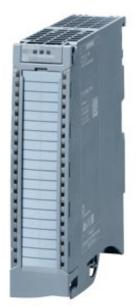
SIMATIC S7-1500, ANALOG OUTPUT MODULE AQ 4 X U/I HF, 16 BITS OF RESOLUTION, ACCURACY 0.1%, 4 CHANNELS IN GROUPS OF 1; COMMON MODE VOLTAGE: 30V AC/60V DC, DIAGNOSIS, SUBSTITUTE VALUE ISOCHRONE MODE, INCL. INFEED ELEMENT, SHIELD CLAMP AND SHIELD TERMINAL
