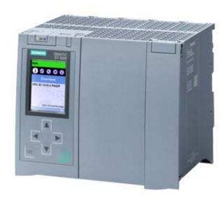
SIMATIC S7-1500, CPU 1518-4 PN/DP, CENTRAL PROCESSING UNIT WITH ODK RUNTIME INTERFACE, WORKING MEMORY 4 MB FOR PROGRAM AND 20 MB FOR DATA, 1. INTERFACE: PROFINET IRT WITH 2 PORT SWITCH, 2. INTERFACE: PROFINET RT, 3. INTERFACE: ETHERNET, 4. INTERFACE: PROFIBUS, 1 NS BIT-PERFORMANCE, SIMATIC MEMORY CARD NECESSARY
